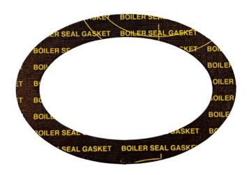
joints in steam processes. Equivalent to the popular Pilot Seal, this gasket has excellent resistance to high temperatures and pressures up to 120°C and 12 BAR, making it a popular choice for steam applications including water heaters, air receivers and paper mill drying cylinders.
