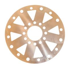
Brasses are divided into two classes. The alpha alloys, with less than 37% zinc, and the alpha/beta alloys with 37-45% zinc. Alpha alloys are ductile and can be cold worked. Alpha/beta or duplex alloys have limited cold ductility and are harder and stronger. CZ108 / CW508L, is an alpha alloy. CZ108/CW508L is a high purity cold forming brass. It is used when severe bending properties are required. It can be machined but only with slow speeds and very light feeds.
