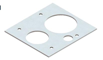
At maximum expansion which occurs at approximately 1200°F (649°C), the paper expands up to 400% of its thickness. This results in the Superwool 607 406-E paper being an excellent candidate for high-temperature gaskets and seals, and fire protection applications. During heat up and expansion, there will be some additional out-gassing of the intumescent additives.
