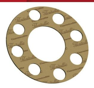
This material is comprised of a tanged 316 Stainless Steel core faced with a high performance vermiculite based sealing material. The metallic core provides improved blow out resistance, handling and cutting characteristics.
